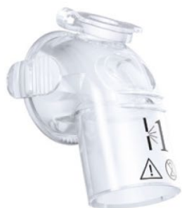
Leak 1 entrainment elbow (EE) click-style has an anti-asphyxia valve for dedicated non-invasive ventilators (use with single-limb circuits)
