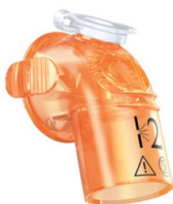
Leak 2 entrainment elbow (EE) click-style has an anti-asphyxia valve for dedicated non-invasive ventilators and intentional leak ports (use with single-limb circuits)
